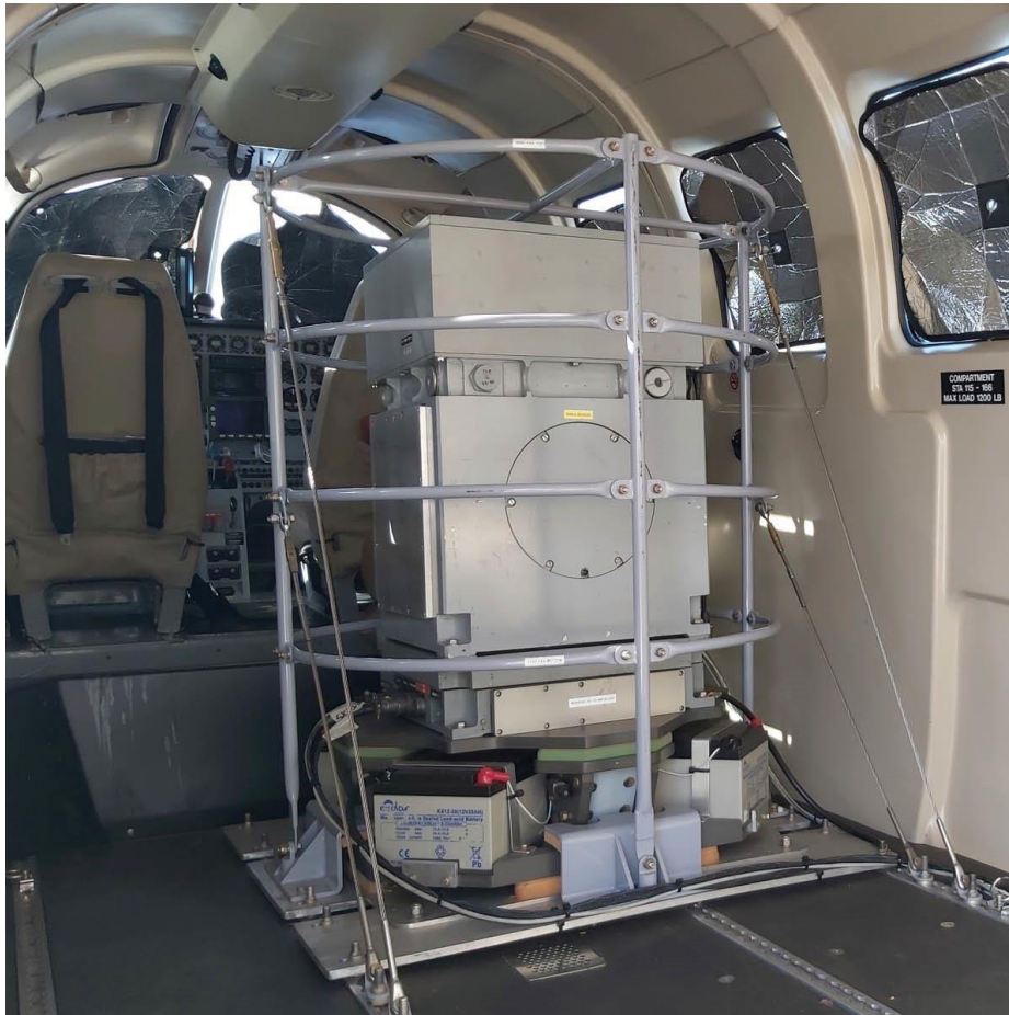
Figure 1. GT-2A Gravimeter installed in the survey aircraft
